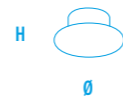
2108/R12 Ø 175 mm H 35 mm Rosone per collegamento da 2 a 12 2108/SM Rose for connection from 2 to 12 2108/SM
